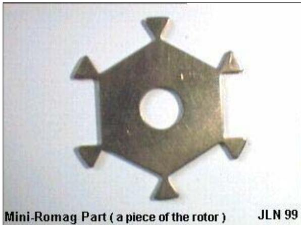
5) Six rotor slots, each 1—3/4" long by .260 deep by 23/32" wide. These slots are spaced exactly 60 degrees apart.
