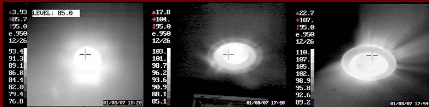
Unsealed down lights & leaking escutcheons
