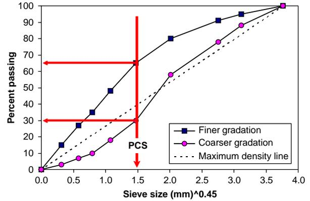
Figure 2. Illustration of the PCS for 12.5-mm NMA5 gradations (coarse and fine).
