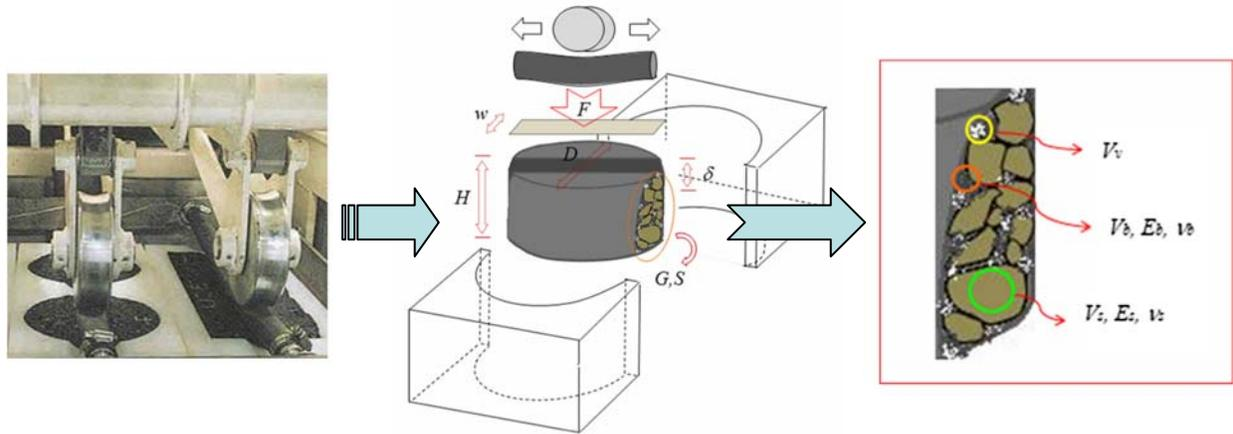
Figure 3. APA testing configuration for the dimensional analysis.
