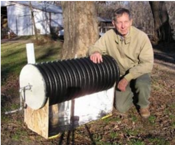
Al Rutan with the digester and warmth chamber
